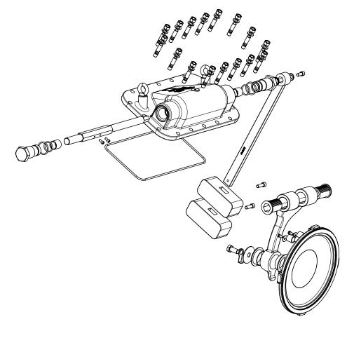
Fig. 6 Head Assembly Components
