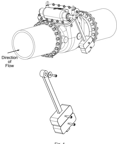
Fig. 4 Lever & Weight Mounting
