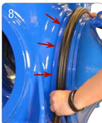
Place the gasket on the connection between valve and center part. Make sure that the gasket is correctly positioned before mounting the brackets.
