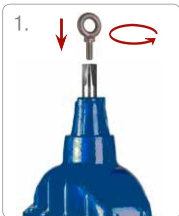
Before dismantling the valve make sure that the system is pressure relieved.
