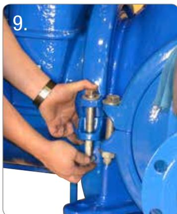
Place the brackets on top of the gasket. Make sure to position the brackets so the air gap is spread evenly between the 2 joints. Bolts can be lubricated with grease.
